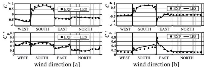
Fig.4: Horizontal distributions of pressure coefficients
