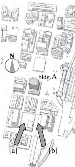
Fig.1: Computed model and wind directions
