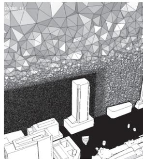
Fig.2: Unstructured grid system
