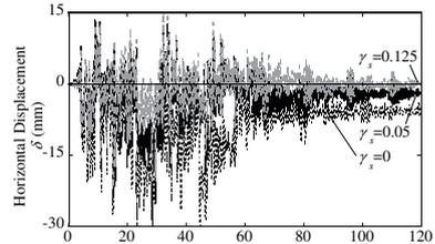
Fig. 4: Displacement of 2<sup>nd</sup> story (2L Model)
