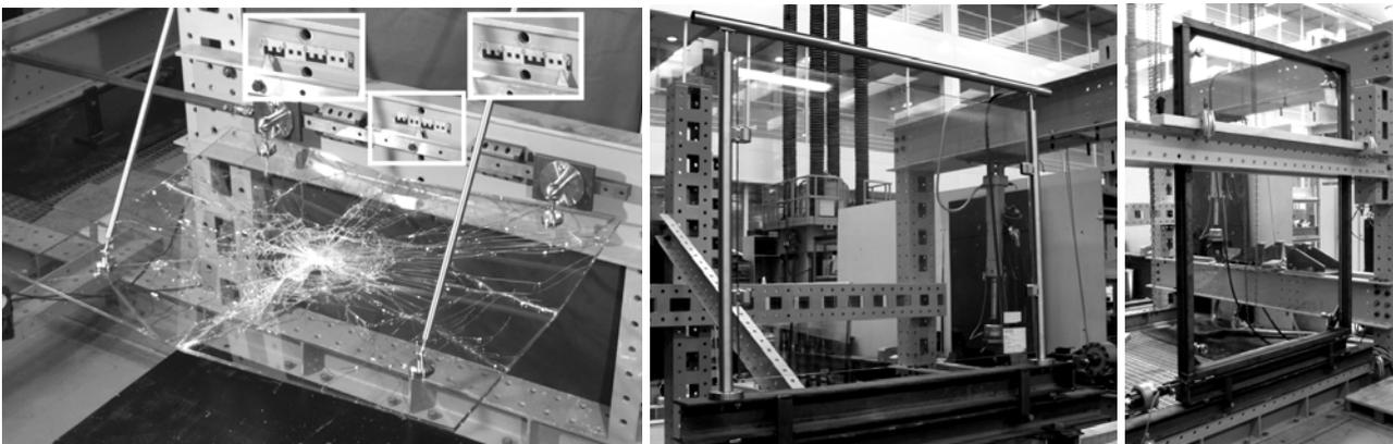
Fig. 5 Test set-ups for earthquake test: canopy, railing and facade element
