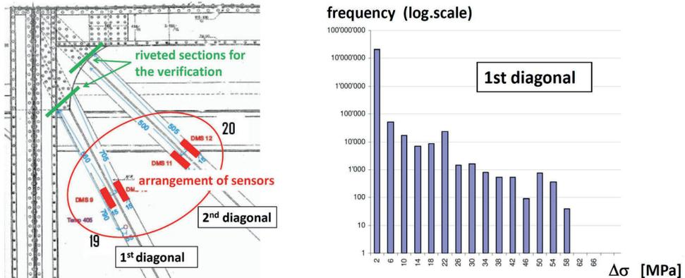
Figure 2: left: location of sensors and verification sections of diagonals of the main truss girder; right: histogram from 12 months of monitoring.
