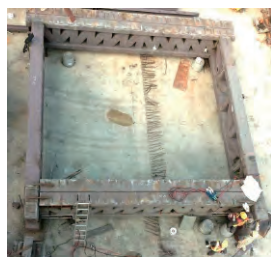
Fig. 5: Crane base frame with twin trusses.
